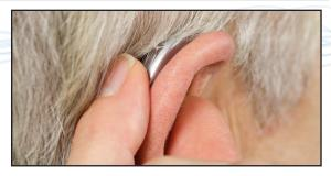
Your Personal Sound<sup>™</sup> allows you to adjust the loudness by briefly depressing the silver Rocker Switch, upward or downward in small steps. A longer press on the switch changes the digital amplifier to the next adjacent listening program. These environmental pre-sets change the basic level and tone property. You can use the volume control function (brief touch) in any of the pre-set programs to achieve your desired level for a given situation.
